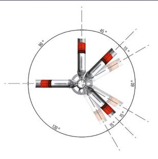
The result of **superior engineering**: up to 8 connections can be made in the structurally ideal Allround Connector, on one level and at various angles.
