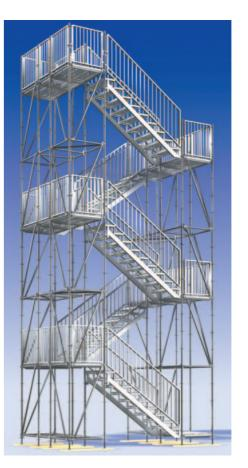
Separate stringers and standard decking ensure variable widths for the stairway (1.09 m, 1.28 m, 1.57 m, 2.07 m). This keeps the weight and the volume of the components low and permits a high proportion of standard Layher Allround material to be used. Local regulations may dictate smaller stair widths than 2.07 m. Please check valid regulations with your local Layher subsidiary.
