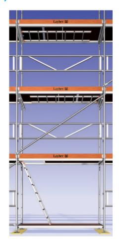
The low-cost variant for upward access in scaffolding: hatch-type decks - with the same function as scaffolding decks comprise work decks, a stiffening element and access inside the scaffolding structure, allowing material to be transported to a limited extent.
